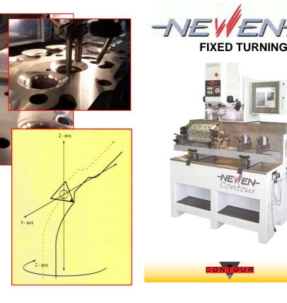
Your valve seats can now be machined on the latest single point CNC fixed turning machining centre.
